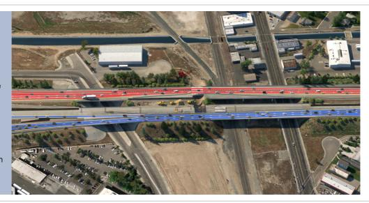
Stage 3: All eastbound traffic will be shifted north onto a temporary bridge near the eastbound lanes of SR 180. During this stage of work, crews will complete the excavation activities and begin construction of a concrete box beneath the highway. Once the concrete box is complete, TPZP will backfill the box and repave the eastbound lanes of SR 180. This stage will last approximately nine months.
