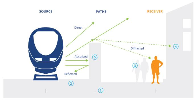
**Above:** The distance (1) between the train tracks and the listener, the type of ground surface (2), ambient noise (3), and the presence of buildings (4) or sound barriers (5) will all influence the noise level that is heard by a listener at any given location
