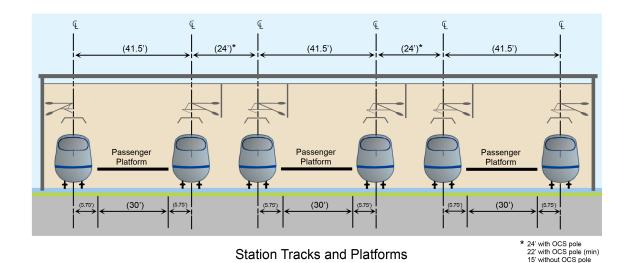
Figure 4-4 Terminal Station—6 Track Terminal and 3 Island Platforms
