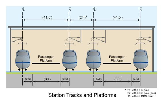
Figure 4-3 Terminal Station—4 Track Terminal and 2 Island Platforms
