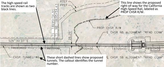
Example 3: Refined CCNM Option - Alignment Drawing - Portion of Drawing Number TT-D1409
