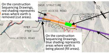
Example 5: CCNM Design Option - Construction Sequencing - Portion of Drawing Number CV-I1101
