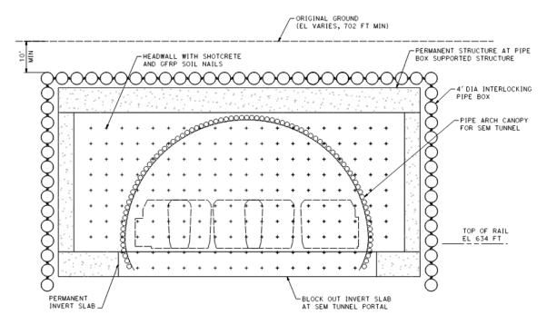
Figure 1. Typical Cross Section of Box Tunnel Excavation with Interlocking Pipes
