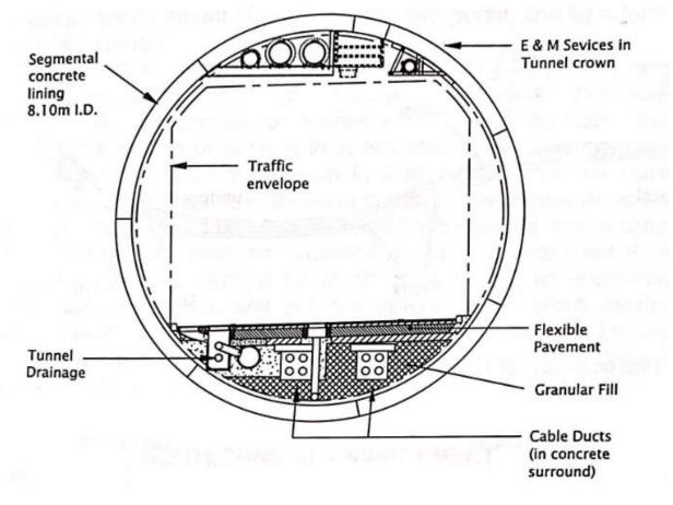
Figure 1-3: Tunnel Cross Section
