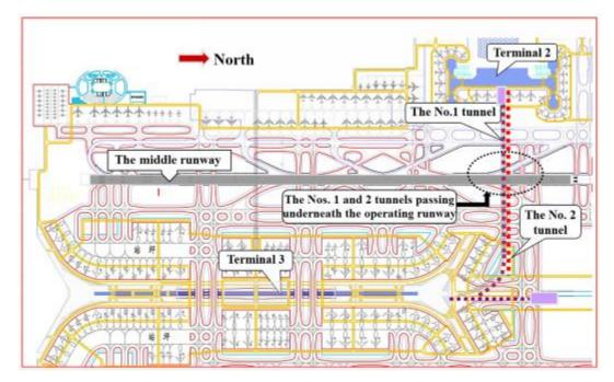
Figure 4-1: Plan of Twin Tunnels and the Middle Runway
