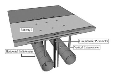
Figure 5-3: Geotechnical Monitoring and Tunneling beneath the Runway
