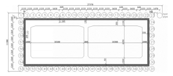
Figure 4-4: Finished Cross Section of the Twin Tunnels and Pipe Layout
