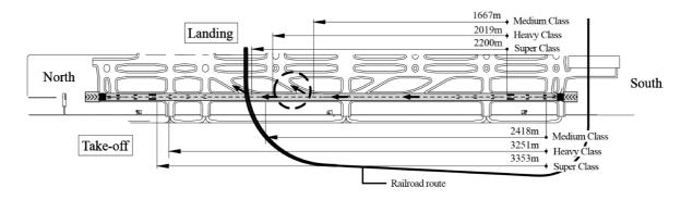
Figure 5-2: Required Distances for Landing and Take-off on Runway
