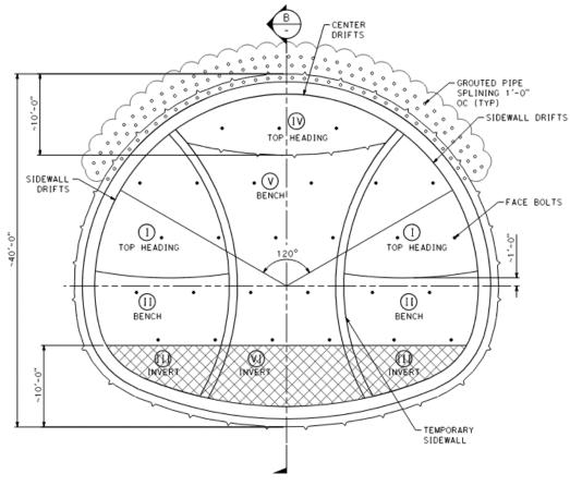
Figure 2. Sequential Excavation Method Construction Sequence
