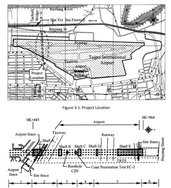
Figure 3-2: Construction Site Plan
