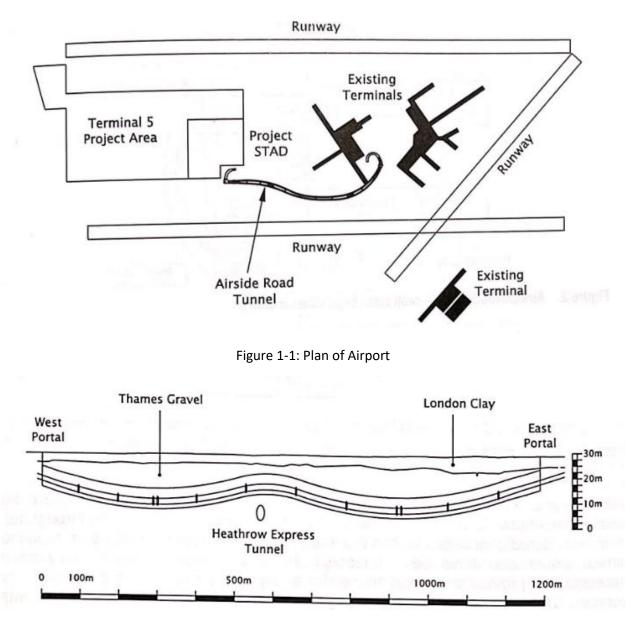
Figure 1-2: Tunnel Longitudinal Section
