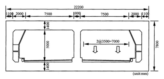
Figure 3-5: Finished Tunnel Cross-section
