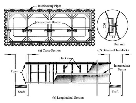
Figure 3-4: Tunneling Sequence
