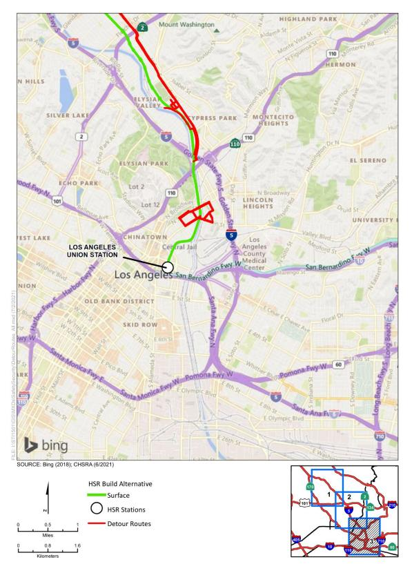
**Figure 3.11-3 Construction Detours**
