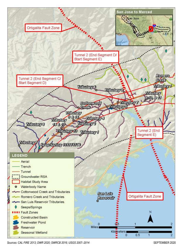
Figure 3.8-15. Groundwater and Surface Water Resources That May Be Affected during Tunnel 2 Construction (eastern portion)
