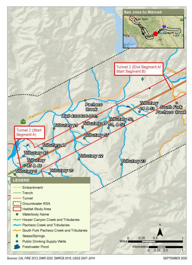
Figure 3.8-13 Groundwater and Surface Water Resources That May Be Affected during Tunnel 2 Construction (western portion)
