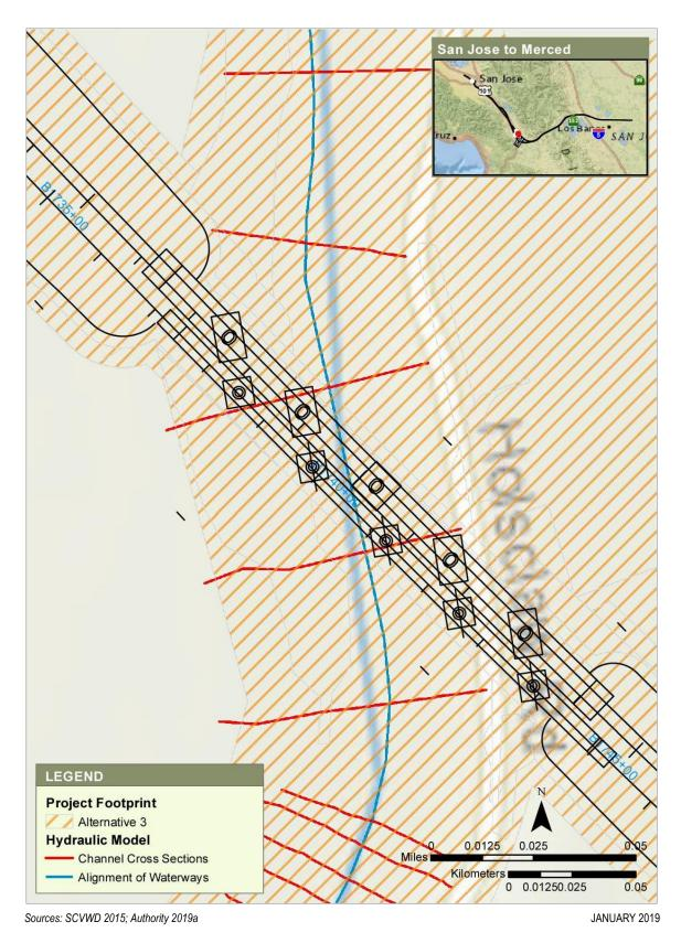
Figure 3.8-16 Hydraulic Model Overview and Proposed Bridge over Llagas Creek near East Gilroy under Alternative 3
