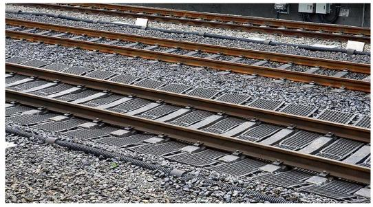
Figure 4-14 Ballast Track with Mats - Japan
