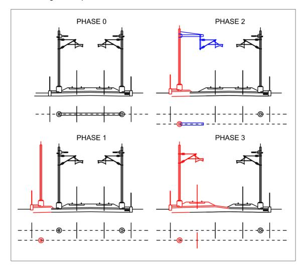
Figure 7. Phases of works for the ascent of the longitudinal profile
