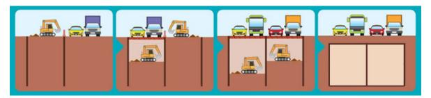
Figure 2. Top – Down Construction Phases
