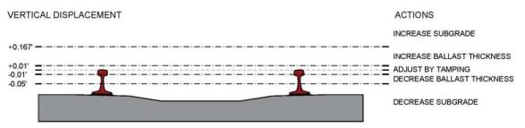
Figure 6. Actions in section for variations in vertical alignment
