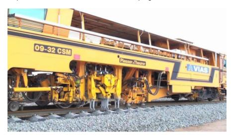
Figure 1. Tamping machine used for lateral displacements of the track between 0 and 1 ft.
