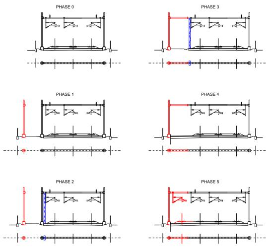
Figure 1. OCS portal beam extension
