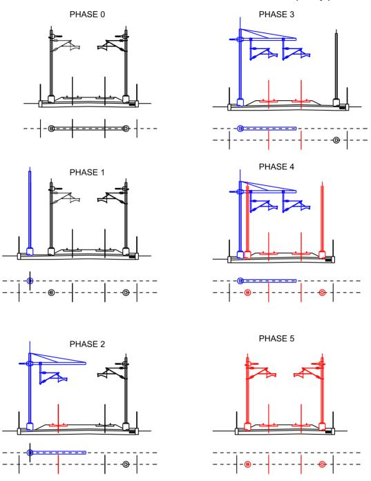
Phase 5: Placement of cantilevers. Removal of the temporary pole.
