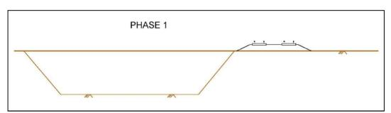
**Phase 1**: Ground excavation adjacent to the structure's permanent location.
