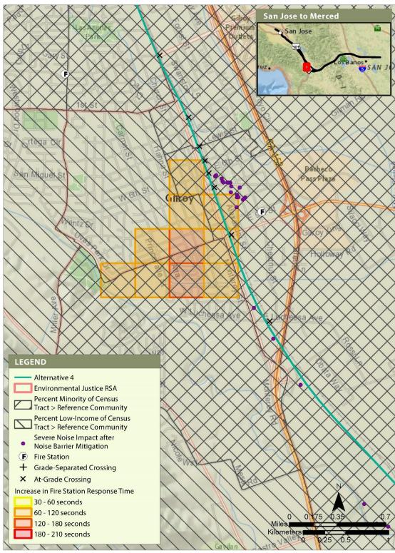
Noise impacts shown are locations of severe noise impacts after noise barrier mitigation (see discussion in Section 3.4, Noise and Vibration).
