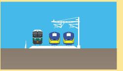
Two electrified, blended service (with Caltrain) passenger tracks and one nonelectrified freight track
