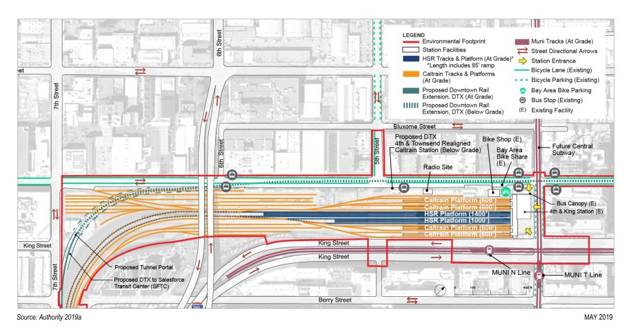
Figure 2-29 4th and King Street Station Site Plan—Alternatives A and B
