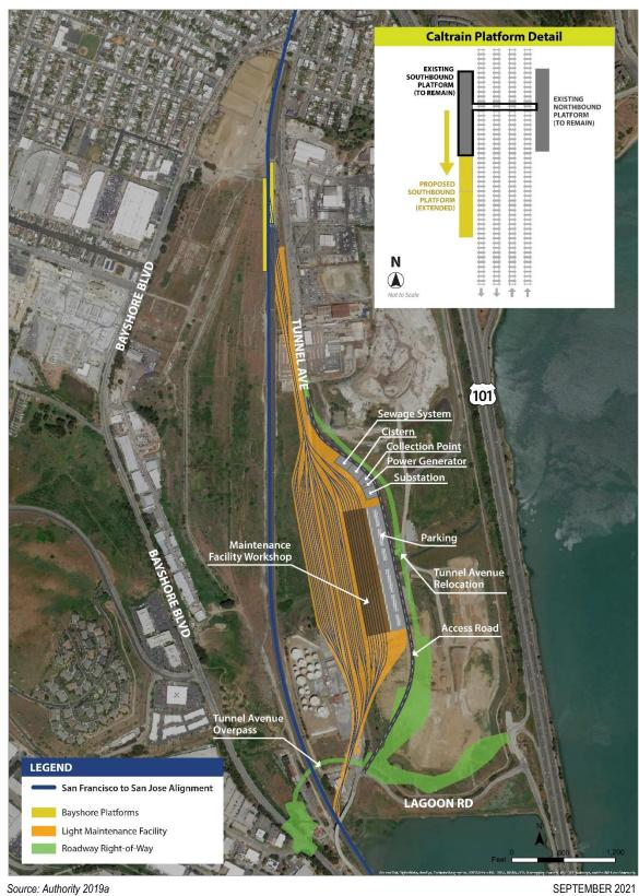
Figure 2-32 East Brisbane Light Maintenance Facility Layout—Alternative A
