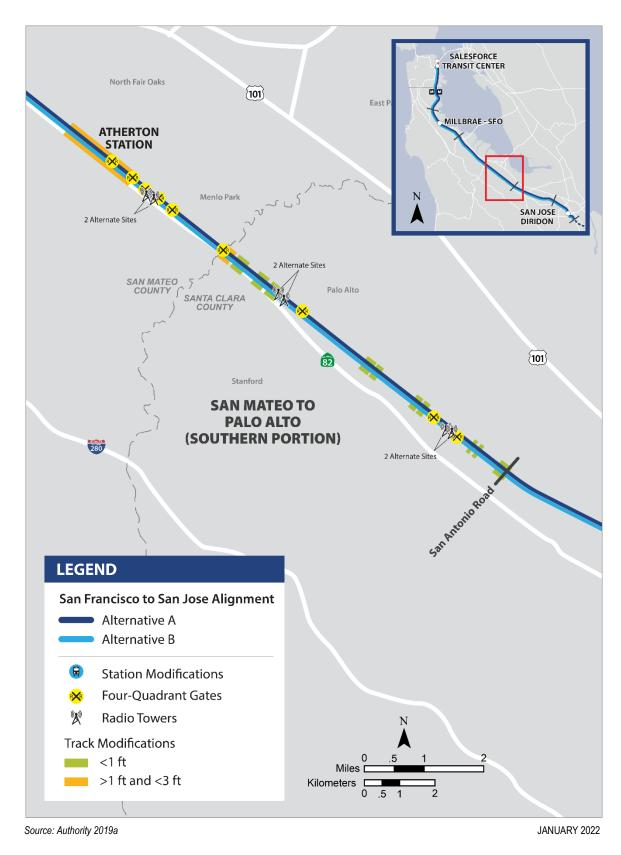
Figure 2-40 San Mateo to Palo Alto Subsection (Southern Portion)—Alternatives A and B
