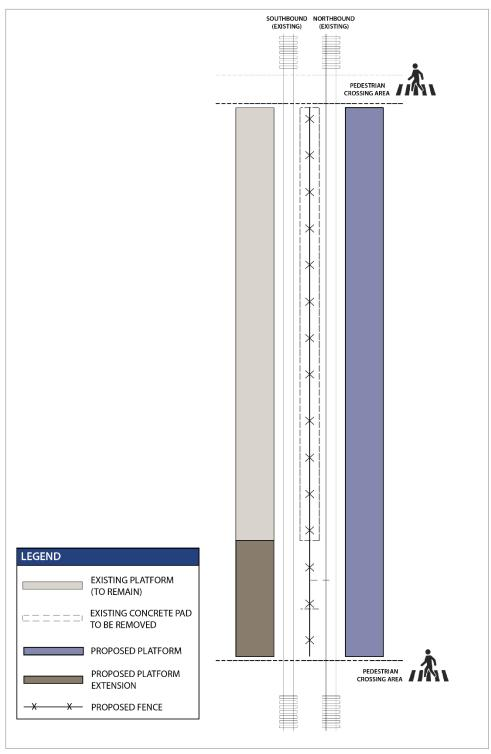
Figure 2-16 Illustration of Hold-Out Rule Stations
