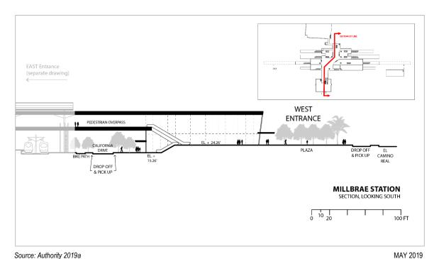
Figure 2-36 Millbrae Station Design Cross Section (West Entrance)—Alternatives A and B
