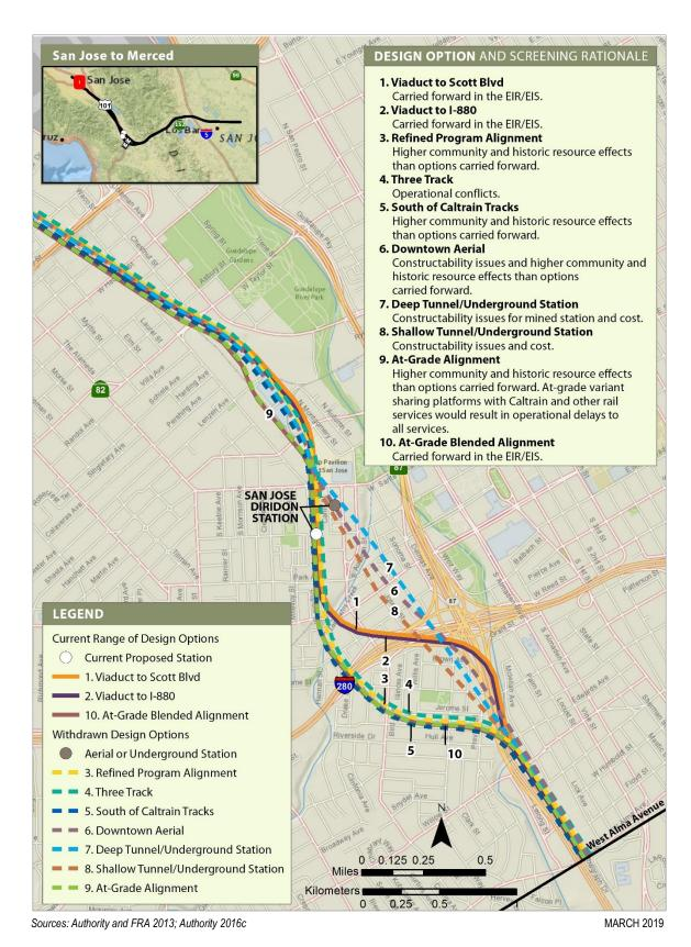
Figure 2-27 Design Options Considered in the San Jose Diridon Station Approach
