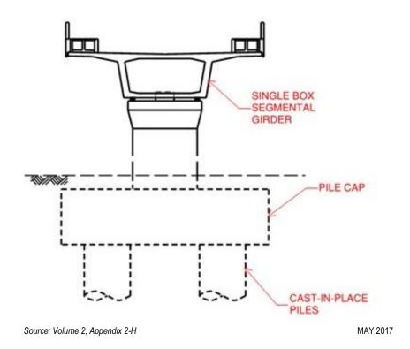
Figure 2-57 Typical Aerial Structure Components
