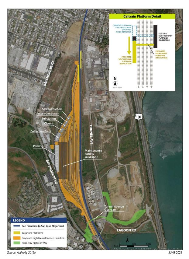
Figure 2-46 West Brisbane Light Maintenance Facility Layout
