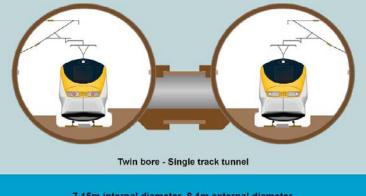
7.15m internal diameter, 8.1m external diameter
