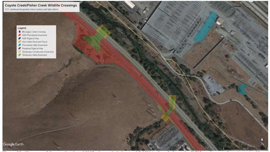
Figure 22. Close-up of Coyote Creek and HSR elevated viaduct and ROW (red) and planned wildlife under-crossings (green) with temporary construction easement estimates (yellow) relative to CCC steelhead designated critical habitat (light yellow line) near Monterey Highway/Old Monterey Highway/Highway 101.
