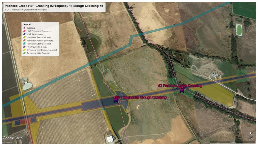
Figure 15. Close up of Pacheco Creek Crossing #2 and Tequisquita Slough Crossing #3 by HSR elevated viaduct/berm and ROW (dark blue) with temporary construction easement estimates (yellow) relative to S-CCC steelhead designated critical habitat in the Santa Clara valley floor (pink line). Electrical interconnections in teal.
