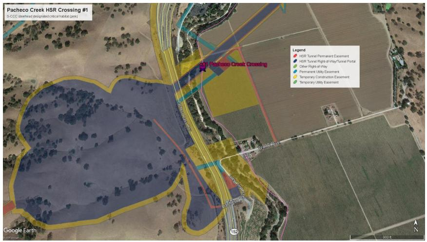
Figure 13. Close-up of Pacheco Creek Crossing #1 HSR elevated viaduct and slope stabilization ROW (dark blue) with temporary construction easement estimates (yellow) relative to S-CCC steelhead designated critical habitat in Pacheco Creek (pink line), just downstream from Casa de Fruta and before tunnel portal transition to second tunnel (red). Electrical interconnections in teal.
