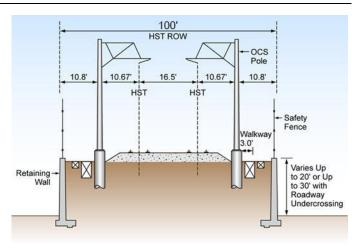
**Figure 2-7** Retained-fill typical cross section
