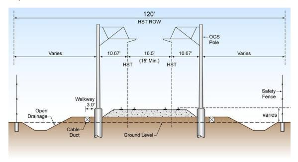
**Figure 2-6** At-grade typical cross section
