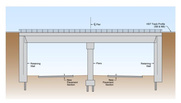
**Figure 2-13** Typical cross section of roadway grade-separated beneath HST guideway
