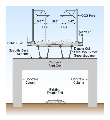
Figure 2-10 Straddle bent typical cross section
