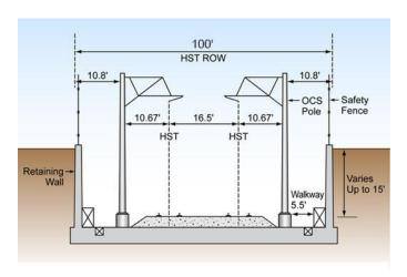
**Figure 2-8** Retained-cut typical cross section
