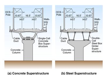
**Figure 2-9** Elevated structure typical cross sections
