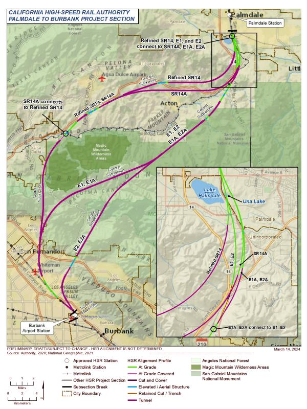
Figure 1-4 Palmdale to Burbank Project Section Build Alternatives
