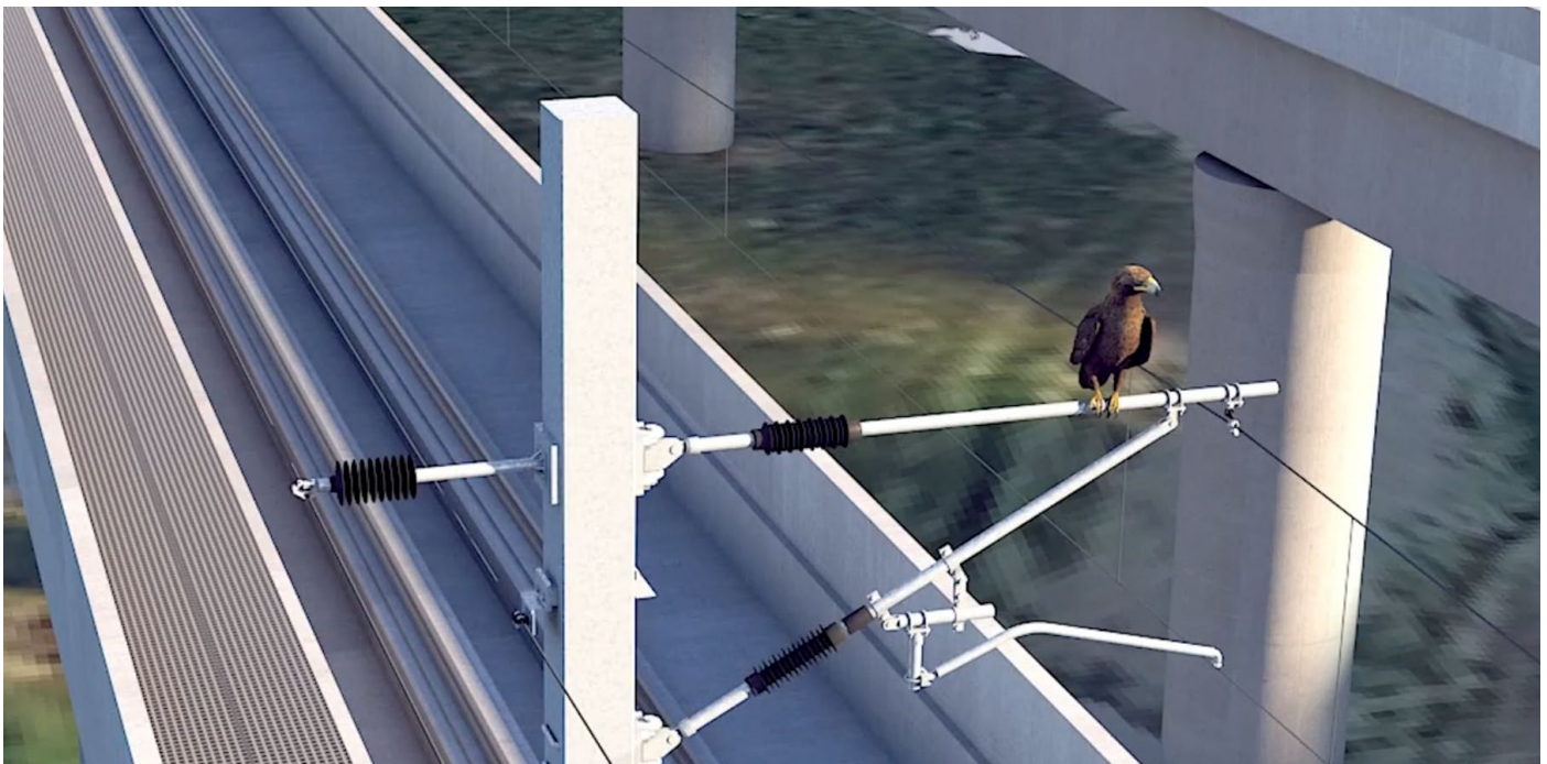
Rendering: The live-loop anti-perching design will keep larger birds safe on the high-speed rail infrastructure.
