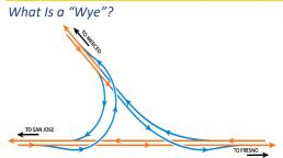
The term wye refers to the Y-like formation that is created at the point where the train tracks branch off the mainline to continue in different directions. eventually decided to carry forward four alignment alternatives for analysis in a supplement to the 2012 Merced to Fresno Final EIR/EIS.<sup>1</sup>
