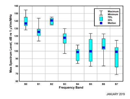
Figure 3 Variation in Measured Maximum Electric Field Strengths
